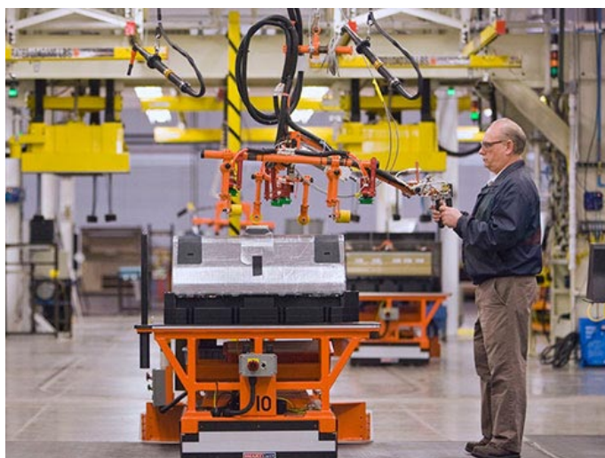
Assembly of a lithium-ion battery in a General Motors plant, USA
